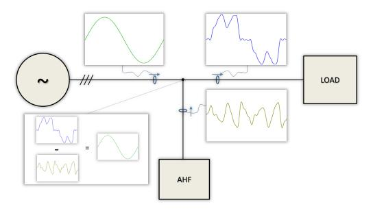
The RHF-Active, and most other active harmonic filter may be used for *pf* correction, unbalance compensation, harmonic mitigation or altogether. It reduces the harmonic current distortion of nonlinear loads and sources to any required *THDi*. This is necessary to reach various standards and recommendations, such as IEEE 519-2014.
